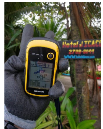
Fig. 5: Coordinates can be taken or environmental elements, such as the image label, can be used to mark the sampling areas. Sampling in Tortuguero, Pococí. September, 2021. Source: CEGESTI (2021).
